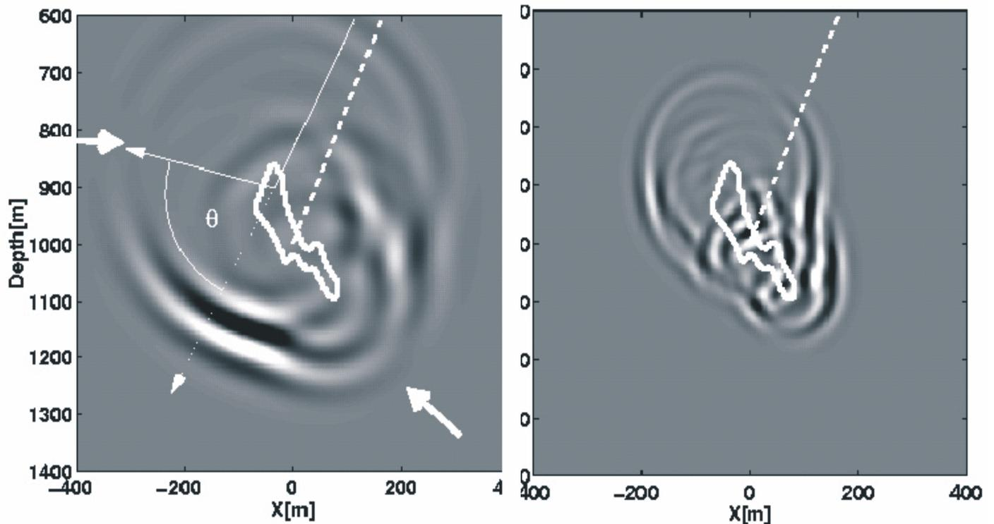
Figure 1. Finite-difference snapshot of scattered P (left) and S (right) waves for a homogeneous background medium of intermediate composition ( $V_p = 6$  km/s) containing a sphalerite inclusion. The shape of the inclusion is modelled after the Bell Allard south orebody in northern Quebec. The dashed line indicates the incident ray direction. Note the single phase reversal (large white arrow) occurring at a scattering angle of approximately 76 degrees. Modified from Bohlen et al. (2003).
